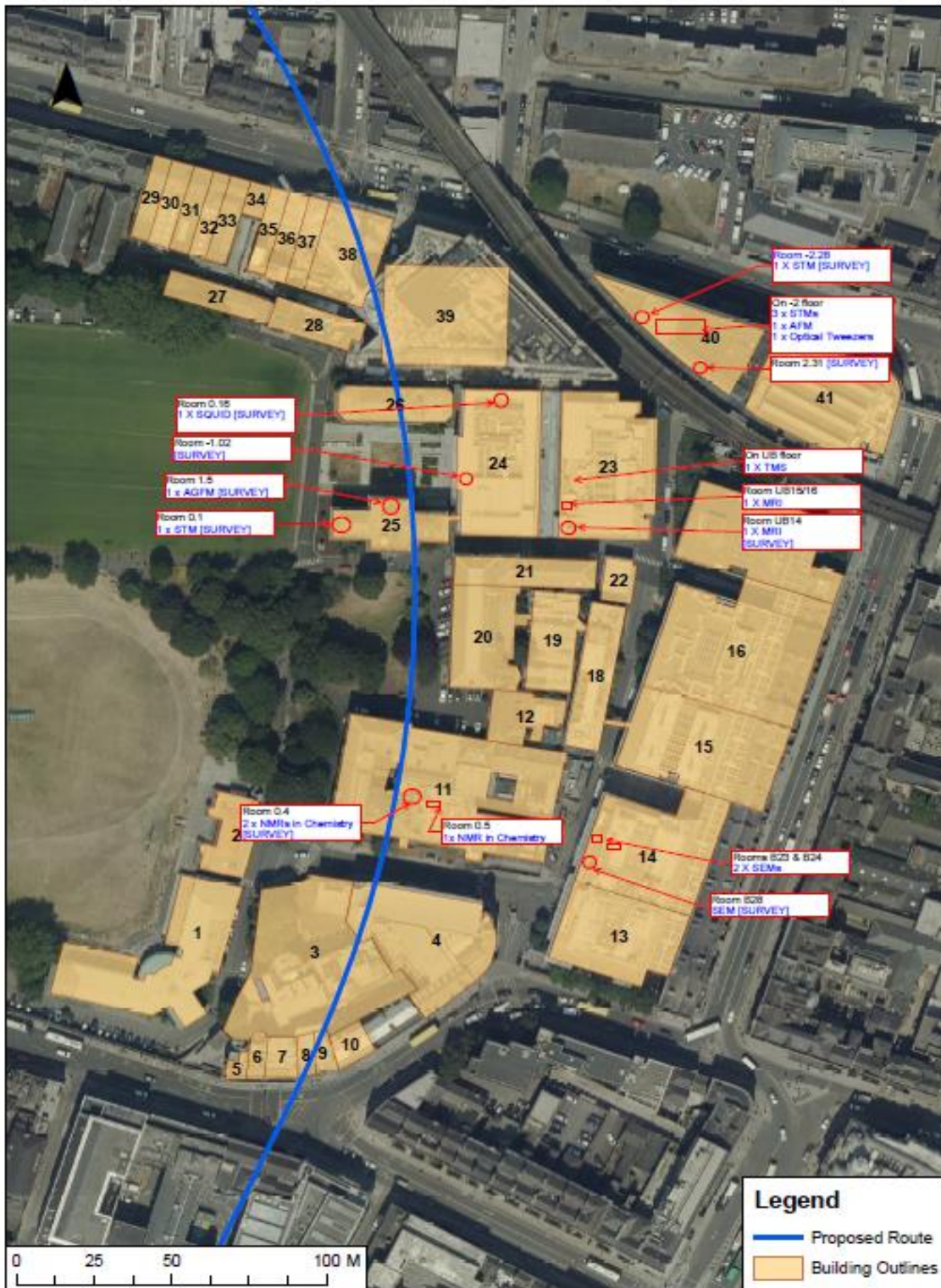
Fig 1.2 TCD sensitive receptors and PDR tunnel alignment
